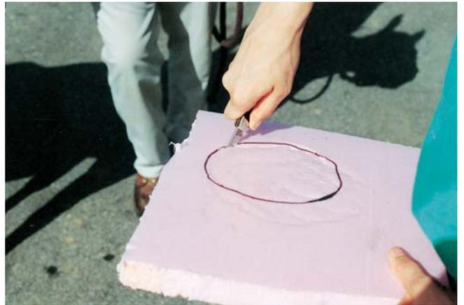
*Fig 4: Fabrication of foam pads. The foot is traced and the pad trimmed with a knife.*
